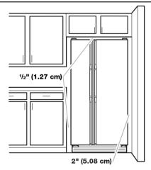
To ensure proper ventilation for your refrigerator, allow for  $\frac{1}{2}$ " (1.27 cm) of space on each side and at the top. Allow for 1" (2.54 cm) of space behind the refrigerator. If your refrigerator has an ice maker, allow extra space at the back for the water line connections. When installing your refrigerator next to a fixed wall, leave a 2" (5.08 cm) minimum space on each side (depending on your model) to allow the doors to swing open.
