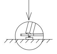
!WARNING! DO NOT LIFT USING GLASS TOP LIFT USING METAL FRAME
