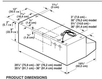
Vent system can terminate either through the roof or wall. Use  $3^{1/4"} \times 10" (8.3 \times 25.4 \text{ cm})$  with a maximum vent length of 35 ft (10.7 m) or 6" (15.2 cm) or larger round vent with a maximum length of 50 ft (15.2 m) for vent system.
