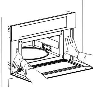
3. Using an 1/8" (3.2 mm) drill bit, predrill pilot holes through the mounting rails on each side of the microwave oven.
