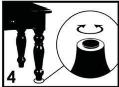
Some furniture come with optional **height adjustment knobs** underneath each leg. Turn this knob counterclockwise to raise the leg level or clockwise to lower the leg level.
