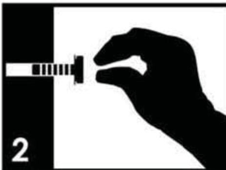
Position each part correctly and insert all screws into their respective holes. Then, **hand-tighten** only until 70% tight. Complete tightening with the tools will come at a later step.
