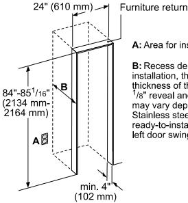
A: Area for installation of power connection.
