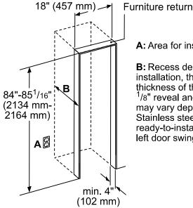
A: Area for installation of power connection.
