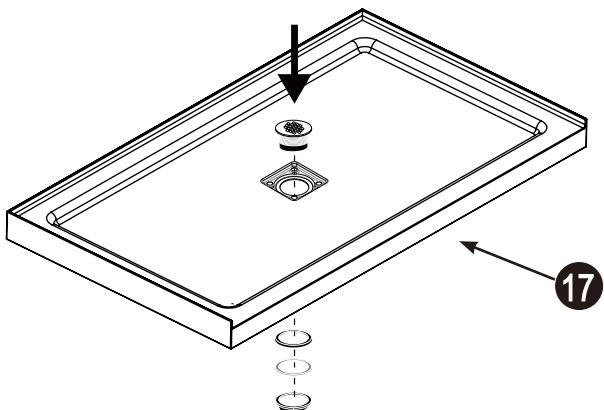
3.1 Place the base (item 17) in its final position. Make sure the base is leveled in each corner. If some studs do not press against the edge of the base, use wood shims to fill the gap.
