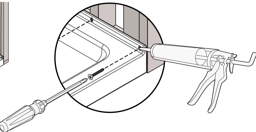
Apply a bead of silicone at the junction of the base (item 17) and the walls and let it sit for 24h.
