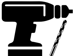
Drill and drill bits Perceuse et forets Taladro con brocas ø1/8" (3mm)
