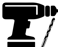
Drill and drill bits Perceuse et forets Taladro con brocas ø1/8" (3.5mm) & ø3/16" (4mm)
