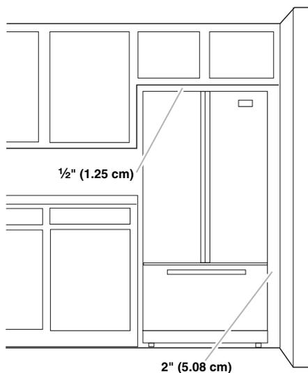
To ensure proper ventilation for your refrigerator, allow for a ½" (1.25 cm) of space on each side and at the top. Allow for a 1" (2.54 cm) space behind the refrigerator. If your refrigerator has an ice maker, allow extra space at the back for the water line connections. When installing your refrigerator next to a fixed wall, leave a 2" (5.08 cm) minimum space between the refrigerator and wall to allow the door to swing open.
